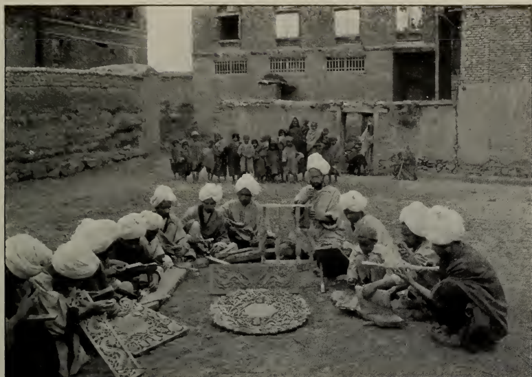
Elaborate woodcarving in Kashmir state, India. A richly decorated stand or table of many vertical supports under construction. Note that each individual is working on a different piece and the foreman is doing the assembling.
